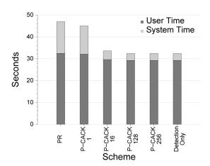
Fig. 12. Sensor processing cost (time to process all packets in a trace), with user and system time breakdown.
