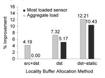
Fig. 5. Percentage of performance improvement when using different locality buffer allocation methods.
