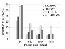
Fig. 18. Utilization of the SRAM memory of the IXP1200.
