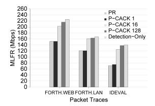
Fig. 14. Sensor Maximum Loss Free Rate (MLFR) using default rule-set.
