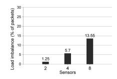
Fig. 4. Performance of CRC16-based load balancing method: difference in percent of assigned packets on most loaded sensor and fair share.
